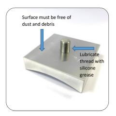
**2**. Apply a small amount of silicone grease to the thread of the lug for lubrication. This will help release the transducer in future if required.
